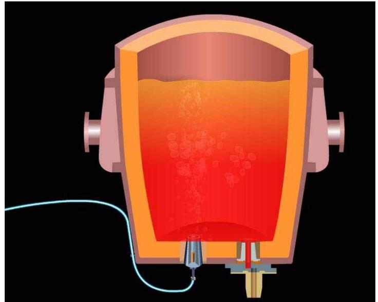
Therefore, it can be concluded that oxygen purging in the ladle can be disastrous for ladle bottom purging.
