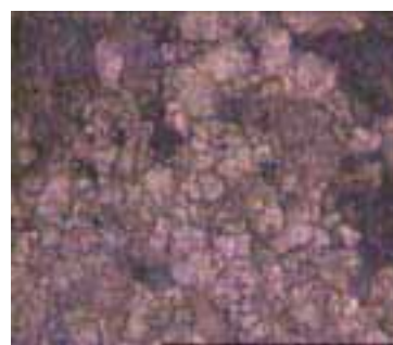
Standard dolomite with 60 micron crystal size
