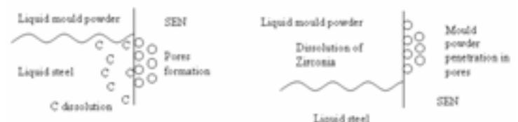
Apart from Carbon dissolution from ZG layer in low carbon steel, some authors have suggested the corrosion mechanism of ZG in steel in a different way. They have reported the formation of ZrC in the ZG layer at low partial pressure of carbon. This ZrC is easily corroded by the penetrating steel and liquid mould powder and the rate of corrosion is further enhanced.
