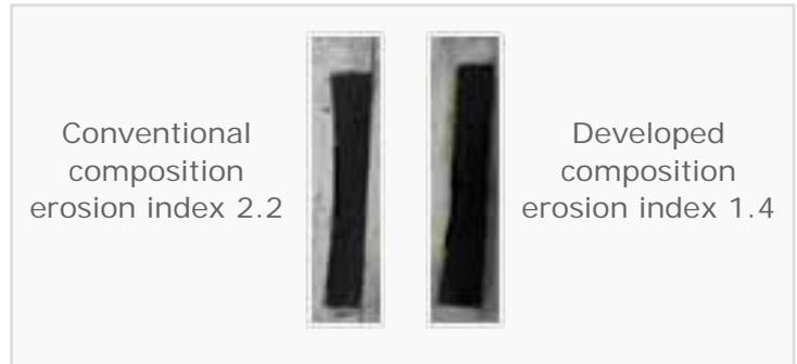
Oxidation resistance test at 1200 °C for 2 hours shows that the oxidation resistance has improved drastically.
