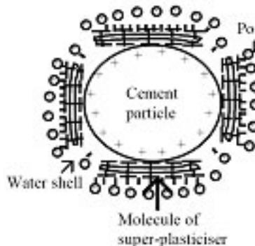
Deflocculants or water reducing agents are absorbed on cement grains, modifying the surface and increasing the zeta potential. Good dispersion occurs due to repulsive effect of the positively charged grains which hamper flocculation.
